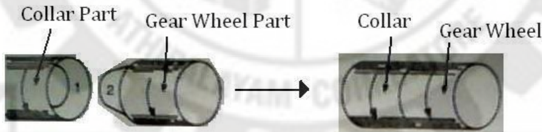
Fig: Two Cones acting as Friction Clutch
