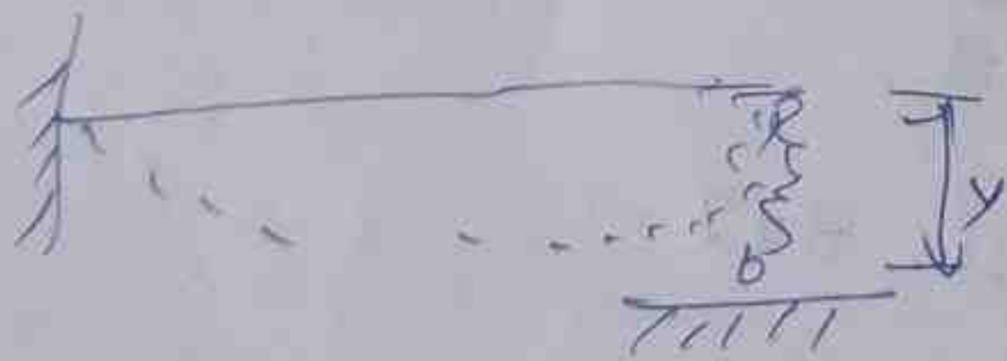
(4) sinking prop (part deflection allowed)
