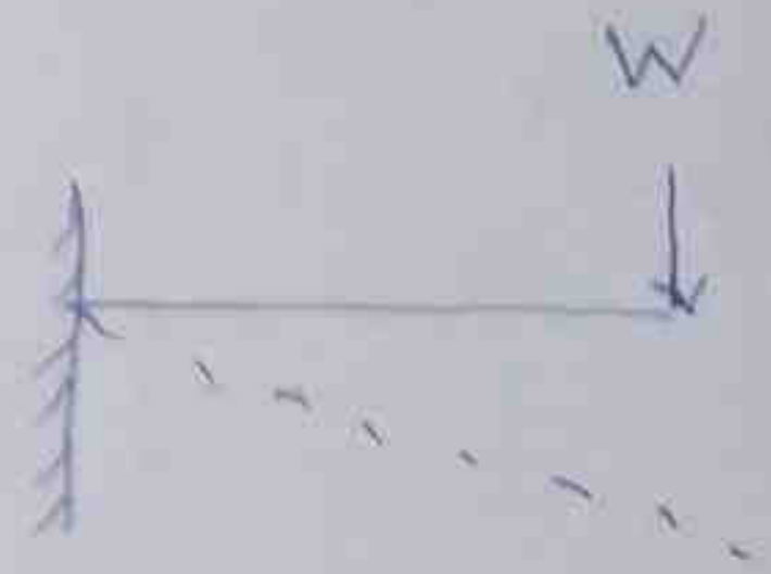
(a) cantilever beam
