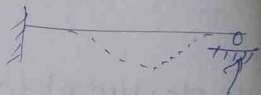
(3) Rigid prop (Deflection at prop is zero)
