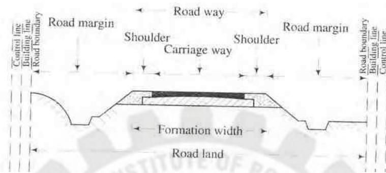
1.3.3.2 (a) Cross section of road in cutting
