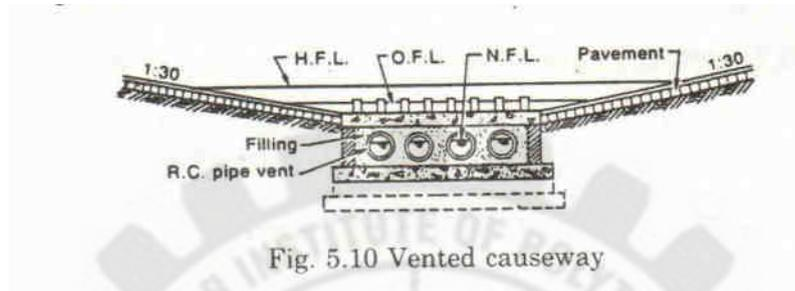
Under the following circumstances Low level causeway or flush cause way is used.
