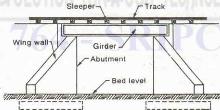
Fig.5.8 Steel girder culvert
