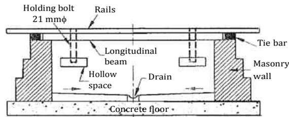
**Fig.4.5 Sectional elevation of ash-pit or Examination-pit**
