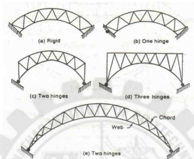
Fig. 5.36 Steel arch bridges
