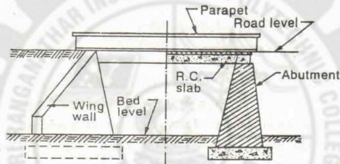
Fig.5.7 Slab culvert
