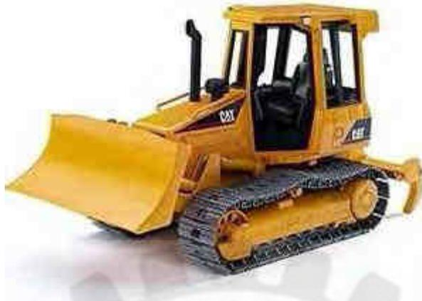
Fig. 2.2.1.1(2) Crawler Type Tractor
