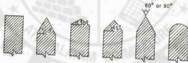
Fig. 5.19 Cut-waters and ease-waters
