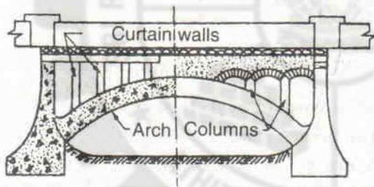
Fig. 5.34 Open spandrel arch bridge
