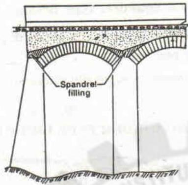
Fig. 5.33 Filled spandrel masonry arch bridge
