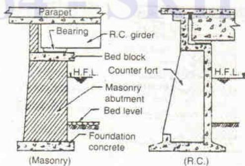
Fig. 5.26 Abutment for girder bridges
