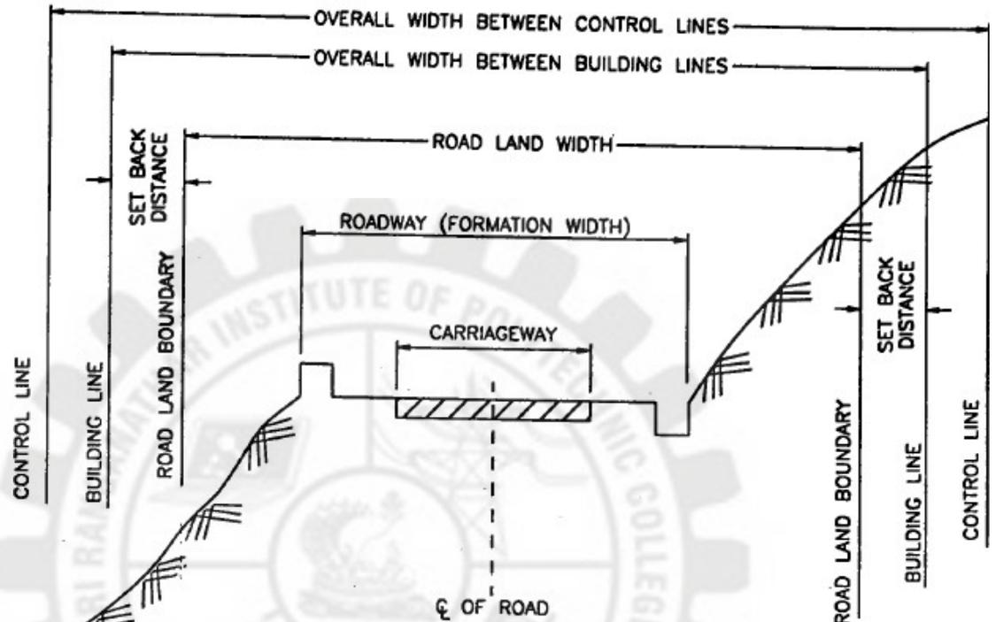
Fig. 2.6.3.1 Cross section of Hill road
