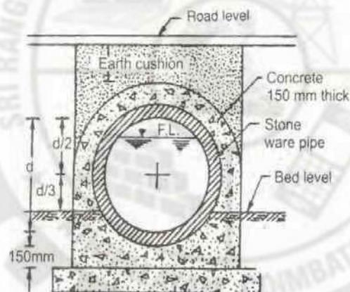
Fig. 5.4 Pipe culvert with stoneware pipe
