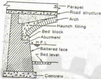
Fig. 5.24 Abutment for masonry arch bridge
