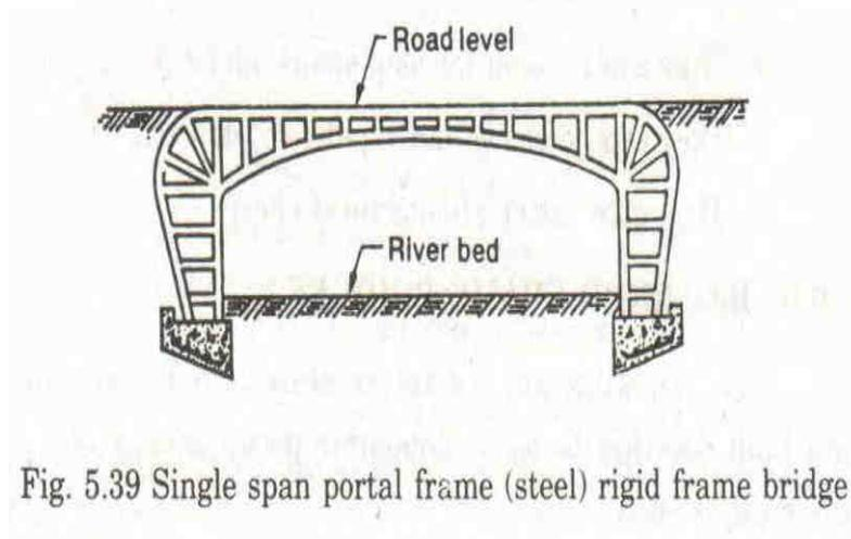
Fig. 5.39 Single span portal frame (steel) rigid frame bridge
