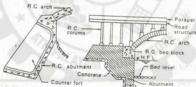
Fig. 5.25 Abutment for R.C. arch bridge
