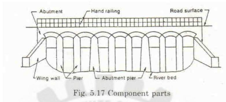
Fig. 5.17 Component parts
