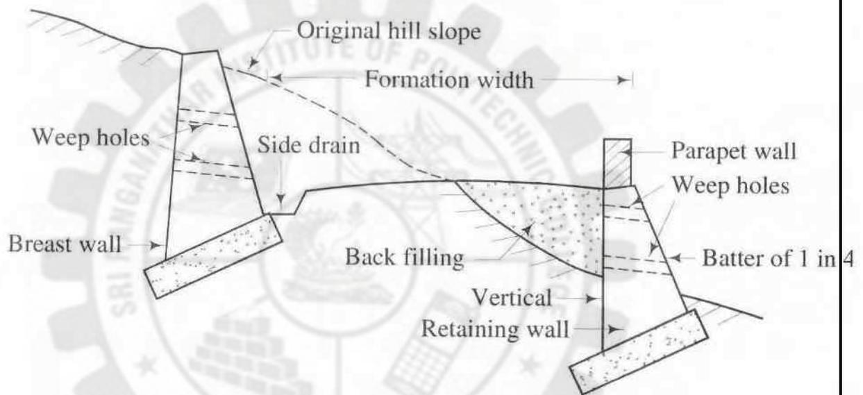
Fig. 2.6.6. Protective works for hill roads
