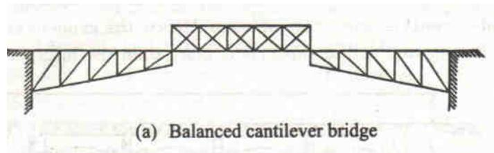
Weight and cross section of cantilevers are determined after trying several possible combinations. The length of cantilever span is  $1/5$  to  $1/3$  of the main supported span.
