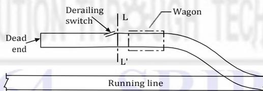
**Fig.4.13 Derailing switch**
