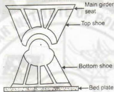
Fig. 5.43 Knuckle bearing
