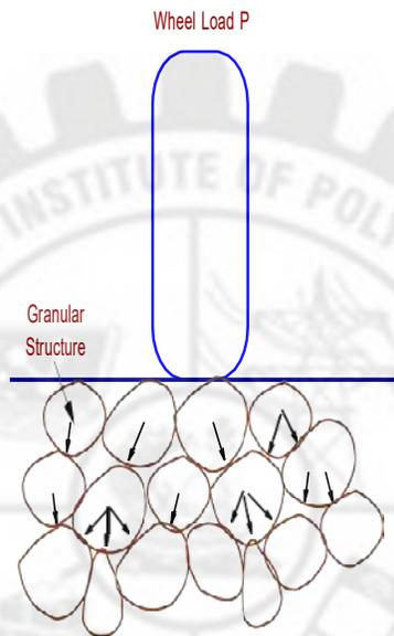
1.2.3 Load transfer in granular structure
