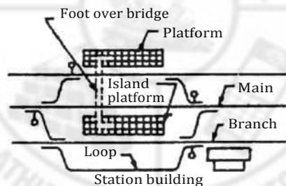
Fig.4.2 Junction station (Layout)
