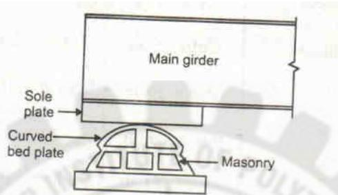
Fig.5.45 Sole plate on curved bed plate
