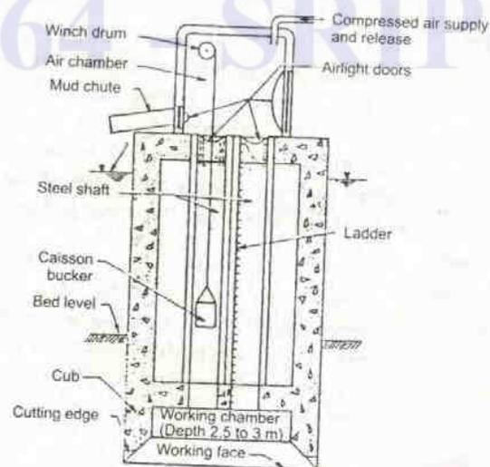
Fig. 5.13 Pneumatic caisson
