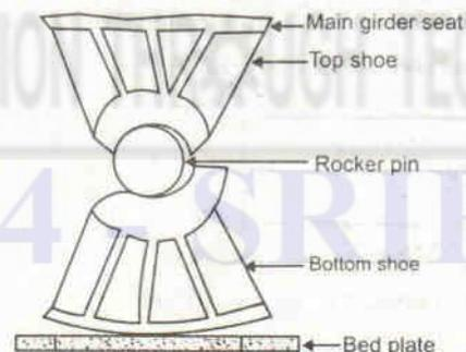
Fig. 5.42 Rocker bearing with curved bottom
