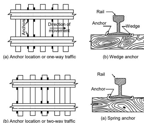
Fig.3.7 Creep of rails -Anchor and location
