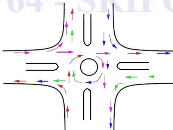
1.4.8.1 (b) Channelization of traffic through a four-legged intersection
