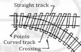
**Fig.4.16 Sleepers for points and crossings - (a) Through sleepers**
