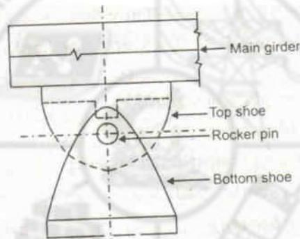
Fig. 5.41 Rocker bearing
