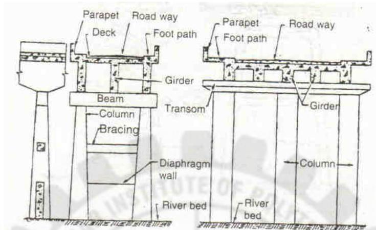
Fig. 5.20 Column bent and column piers
