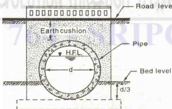
Fig. 5.2 A pipe culvert
