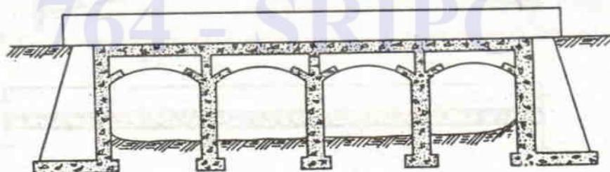
Fig. 5.30 Continuous bridges (R.C.)
