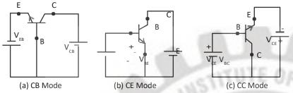
The term common is used to denote the lead that is common to the input and output circuits. The three different modes are shown above for NPN transistor .
