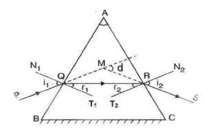
• ABC is an equilateral glass prism, AB, AC are the refracting faces. BC is the base of the prism
