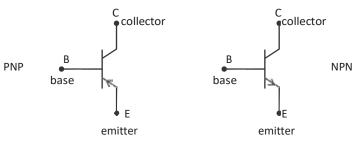
In the symbolic representation for a transistor, the arrow mark is placed on the emitter in the direction of conventional current flow, i.e., from P to N direction.
