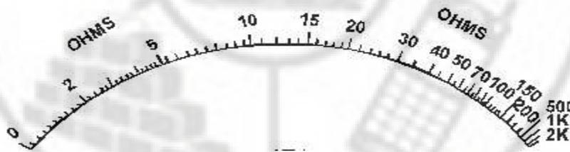
Fig.2.20 b. Scale of Shunt type ohmmeter
