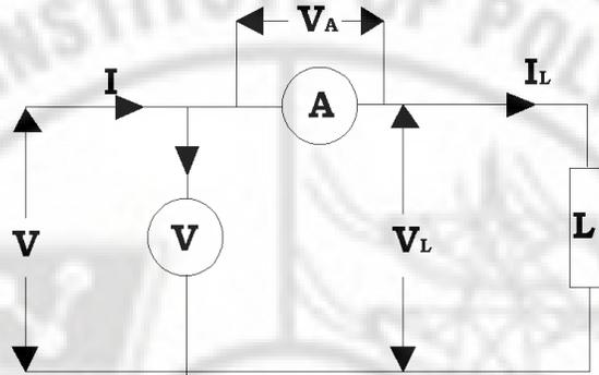
**Fig. 3.1 b. Power measurement in DC circuits**
