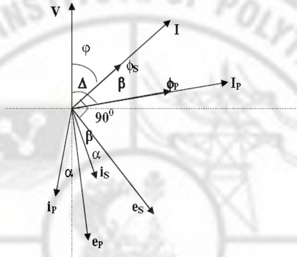
**Fig2.5 b. Vector diagram of Shaded Pole Instrument**
