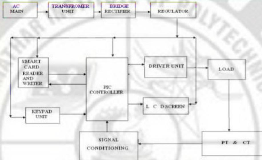
**Fig.3.21. Block Diagram of a Digital Energy Meter**
