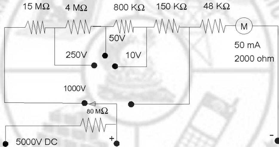
**Fig.2.25. Multimeter for Measuring Voltages**
