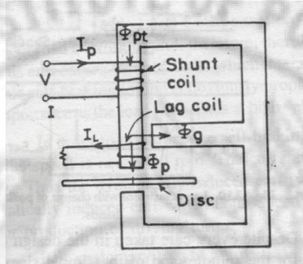
**Fig. 3.12. Shading coil with low resistance for phase displacement error correction**
