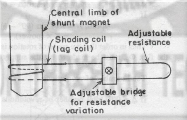
**Fig. 3.13. Shading band**
