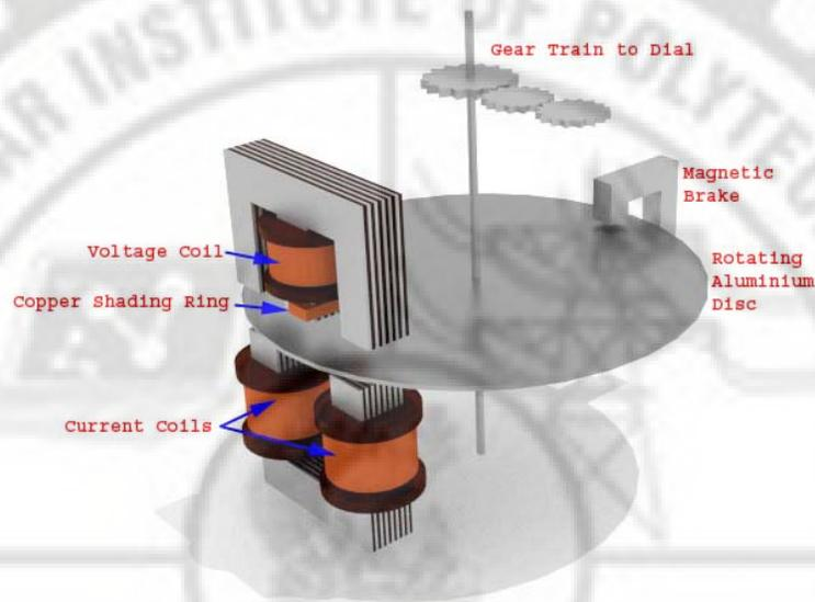
**Fig.3.10 c. Dimensional view of Single Phase Induction Type Energy Meter**
