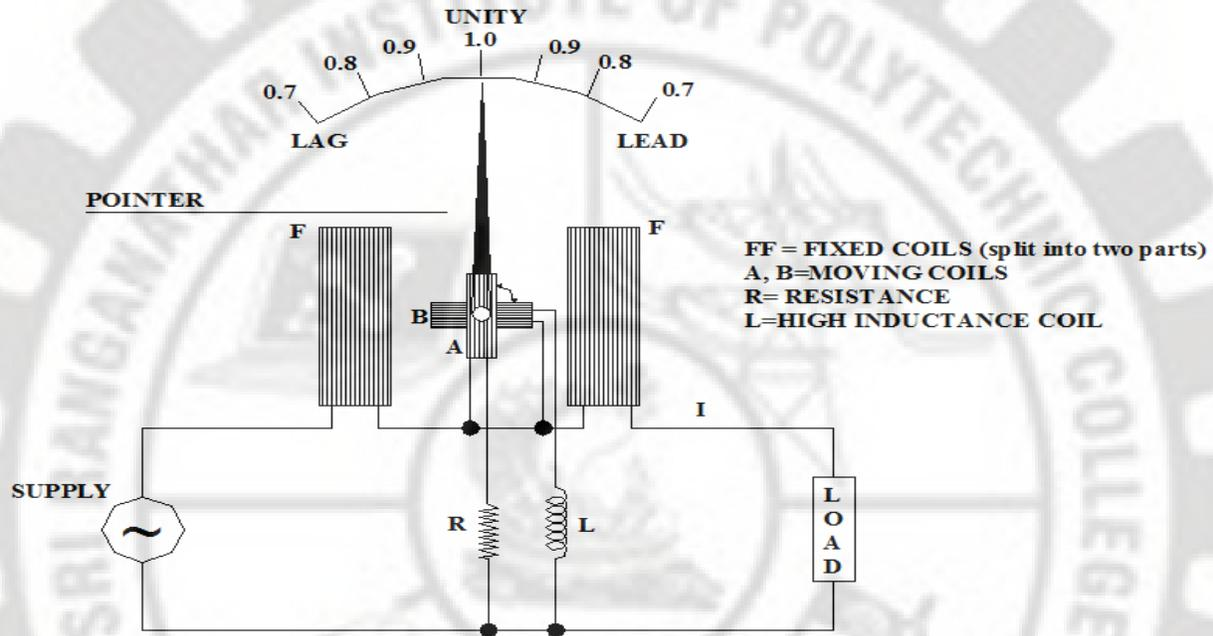
**Fig 4.1.single phase power factor meter.**
