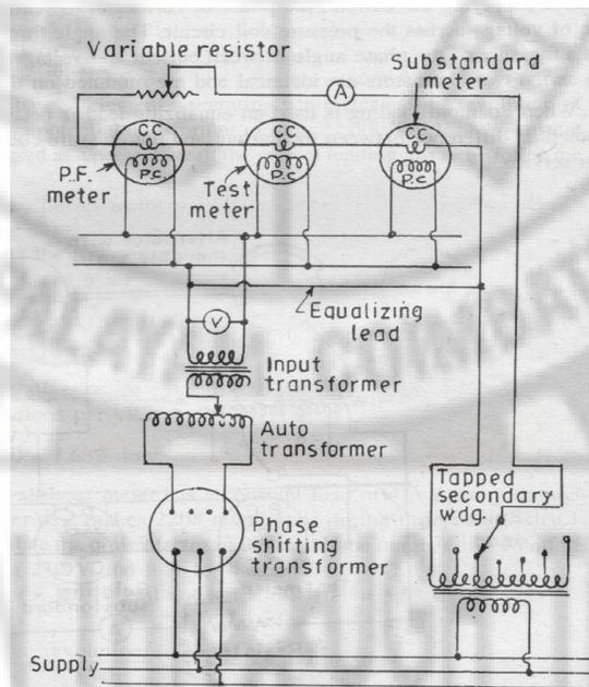
**Fig.3.20. Calibration of energy meter using RSS meter**
