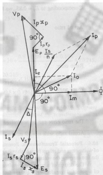
Fig.2.16 Vector diagram of a PT
