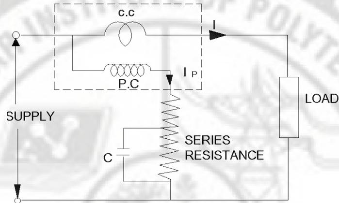
Fig.3.6 Low Power factor wattmeter
