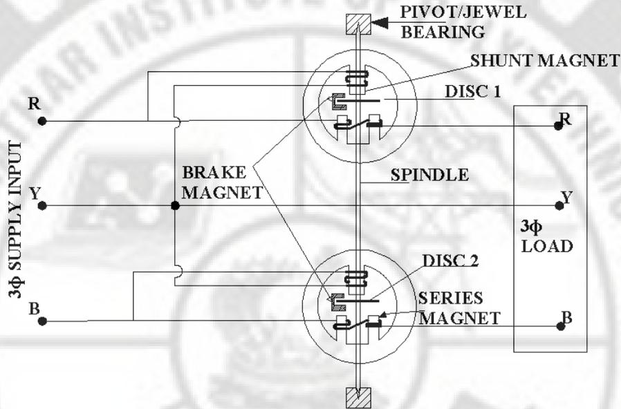
**Fig.3.19 Two Element Three Phase Energy Meter**
