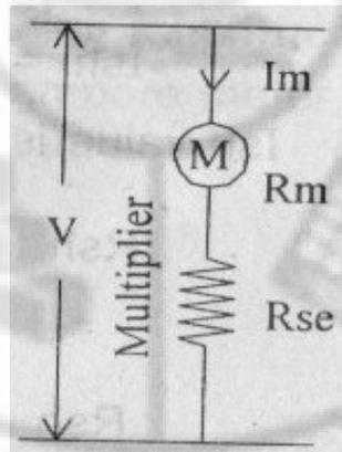
**Fig2.10 Extension of voltmeter range by multiplier**
