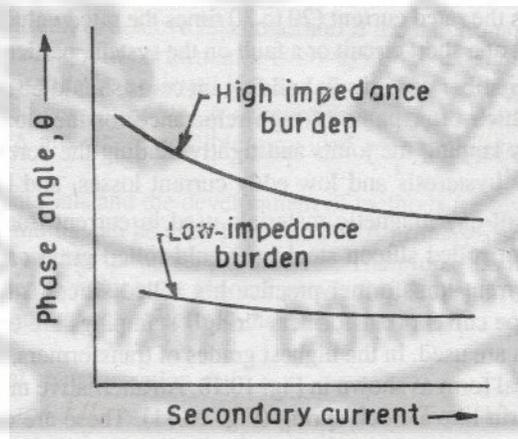
**Fig.2.15 b. Variation of phase angle error with secondary current**
