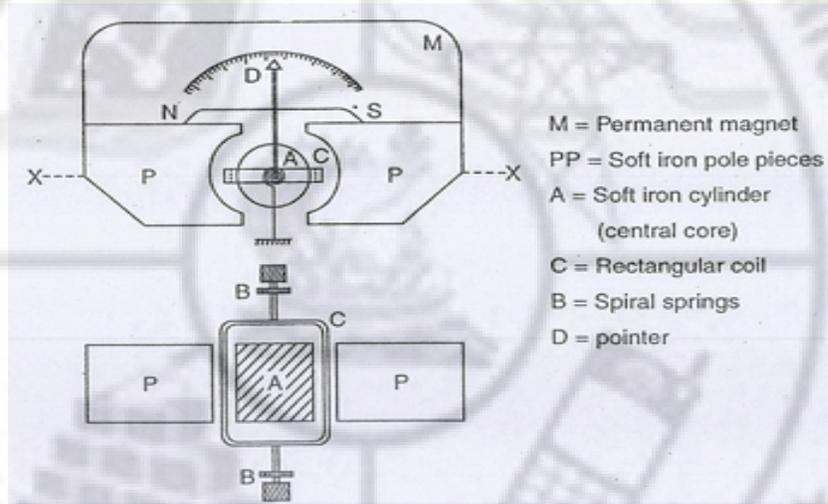
**Fig 2.1 PMMC Instrument**
