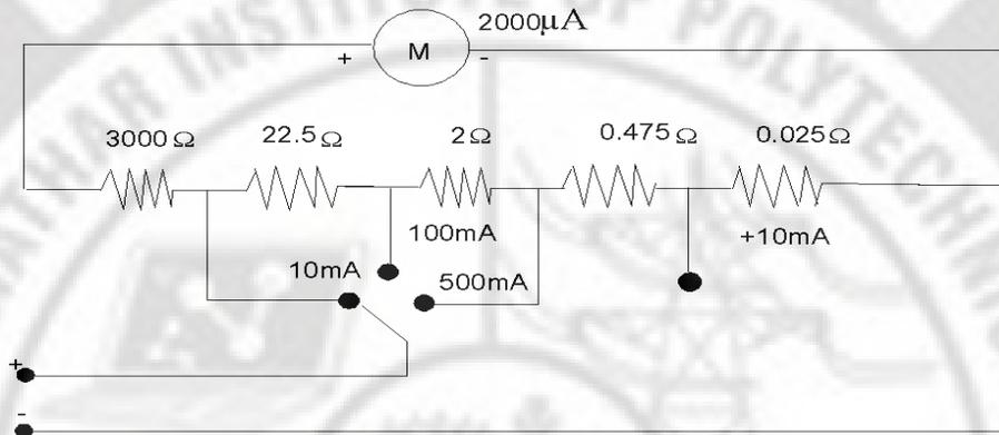
**Fig.2.26. Multimeter for Measuring Currents**
