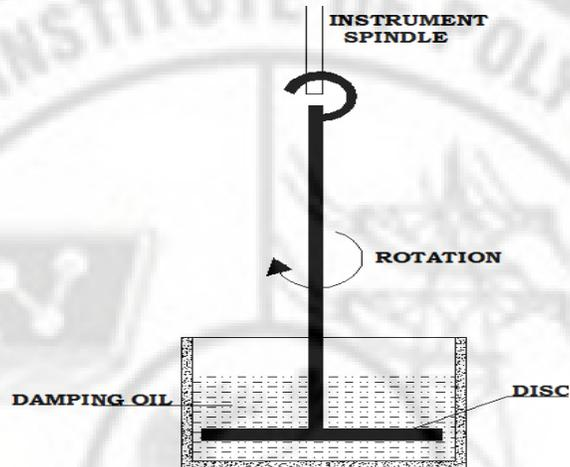
**Fig 1.8 Fluid Friction Damping**
