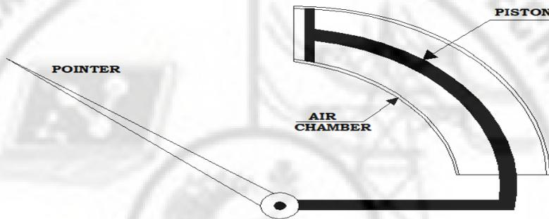
**Fig 1.7 Air Friction Damping**
