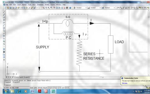
**Fig. 3.4 Compensation for power loss in pressure coil circuit**
