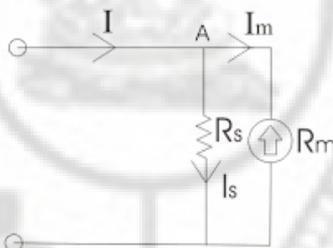
**Fig2.9 Extension of Ammeter Range By Shunt**
