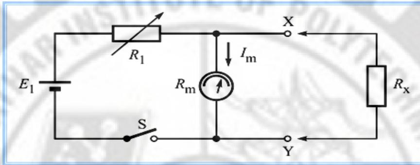
Fig.2.20 a. Shunt type ohmmeter
