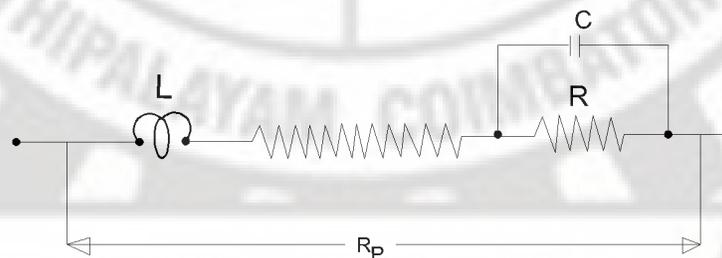
**Fig 3.5. Compensation for inductance of pressure coil circuit**
