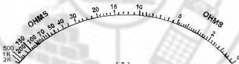
Fig.2.21 b. Scale of Series type ohmmeter
