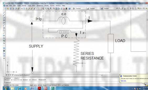
**Fig.3.3 b. Wattmeter connections**
