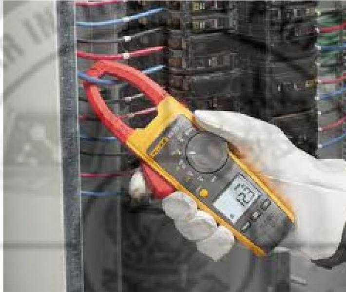
**Fig2.11 b. Measurement using Tong Tester**
