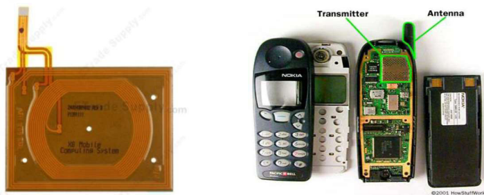
Figure 5.7 Battery and Antenna
