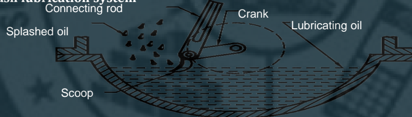
Fig.8.28 Splash lubrication system
