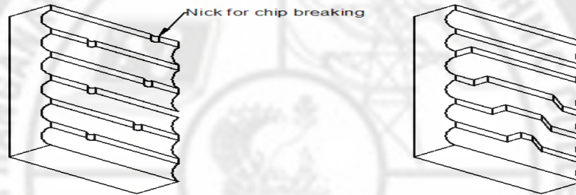
Fig. 2.41. Solid Broach and Progressive Broach
