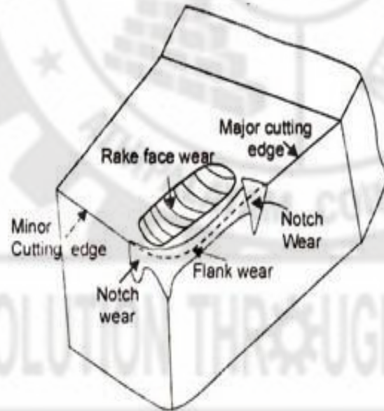
Fig. 9.16. (a) Tool Wear Phenomena.
